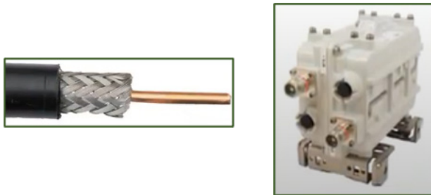
Figure 4: Internal PIM sources
